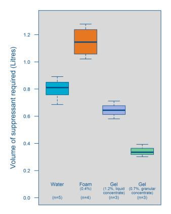
Figure 2. Plots showing the normalised distribution of the volume required for the extinction of standard fires using some example suppressants.
